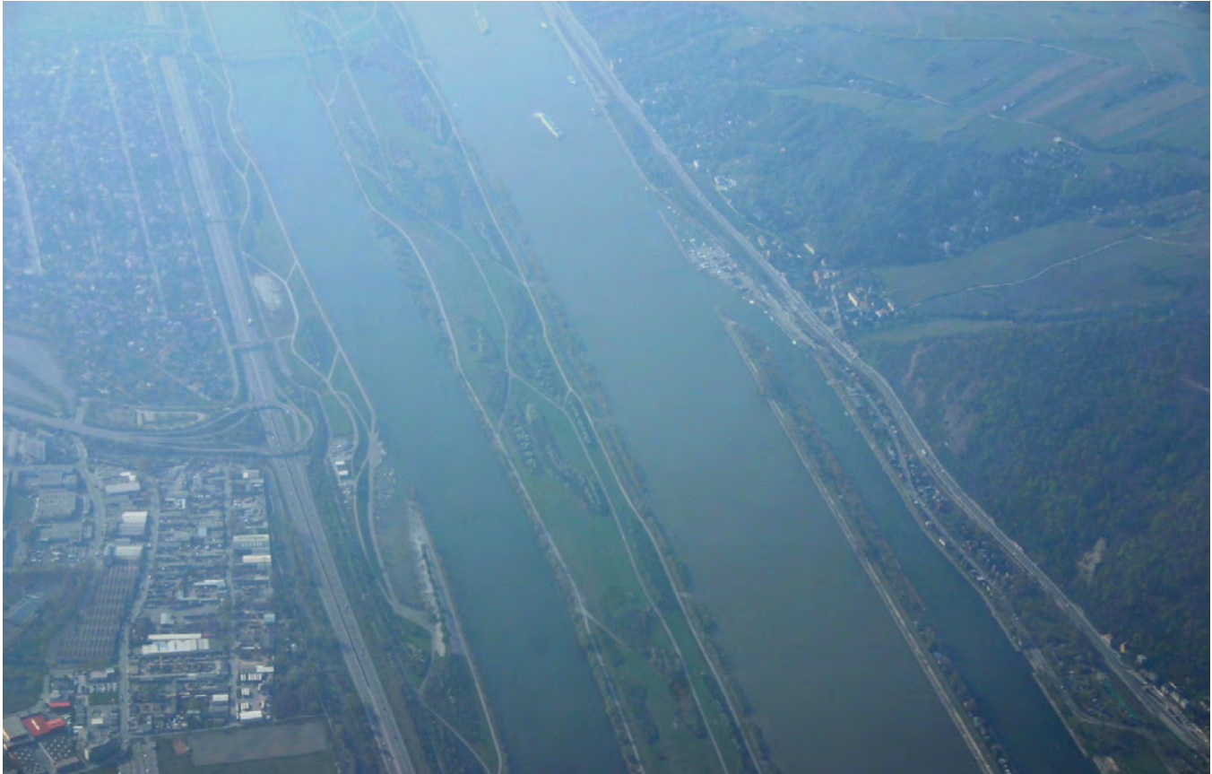
Photo 6.8 Donau River and canal downstream from Vienna, Austria have been straightened to improve navigation. New measures have been taken to restore the natural flood channels of the river in the Donau-Auern National Park. © Roger Crofts
